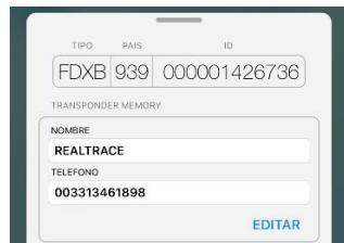
**ISO FDXB tag compatible with the possibility to write additional data A name and a phone number to datachips Application PetScan on iPhone and Android**
